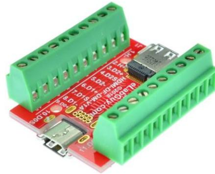
Figure 4: HDMI-DF-DF-V1A with terminal blocks
