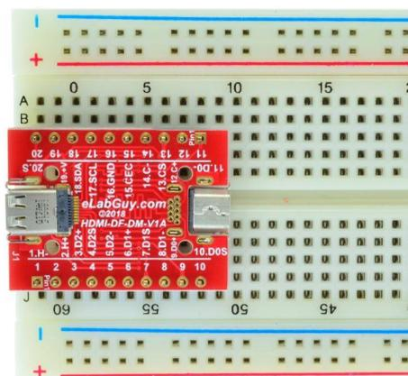
Figure 2: Example of connecting the HDMI-DF-DF-V1A on a proto PCB (Note: This picture only shows the pins spacing, actual use may not be used on a breadboard)
